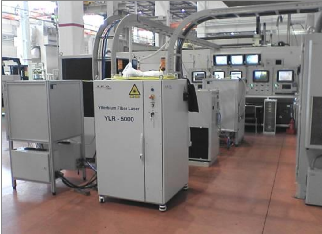
Tailored Blank Schweissanlage P=5kW, v=12m/min, s=0,8-1,4mm
